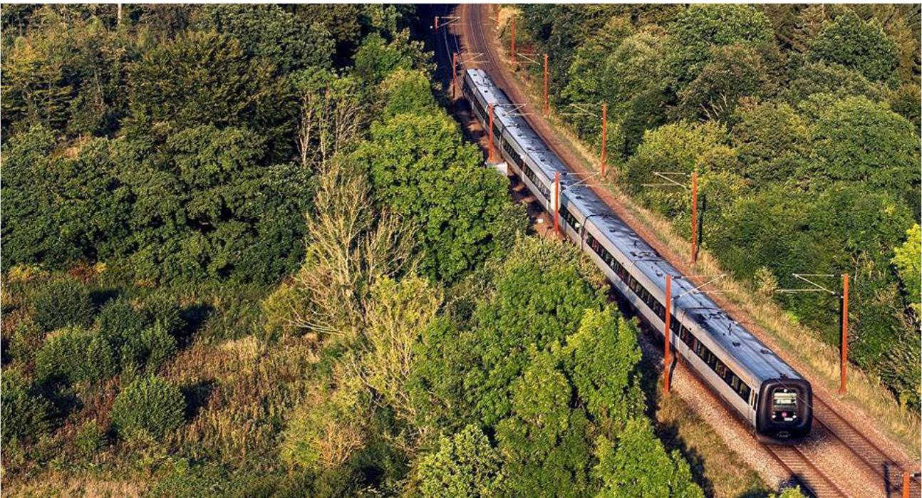
OLE on a railway in Denmark, using weathered steel masts (photograph: © Network Rail)
