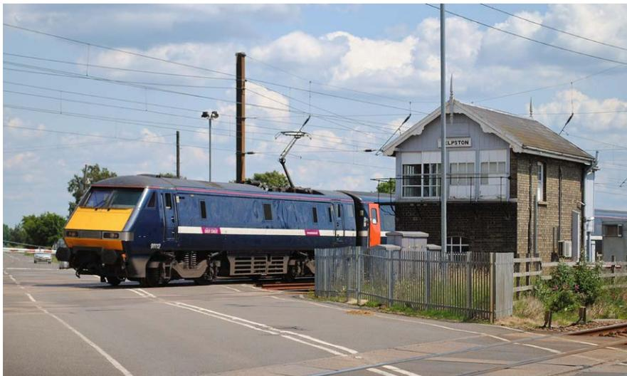
Level crossings - note how the pantograph on the train is extended to reach the raised contact wire (photograph: © Philip Hilbert)
